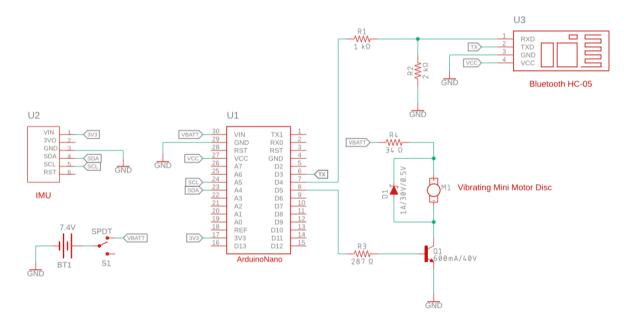
Figure 11: Schematic Diagram of the Hardware Device
