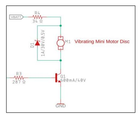
Figure 13: Vibrating Motor Module Schematic
