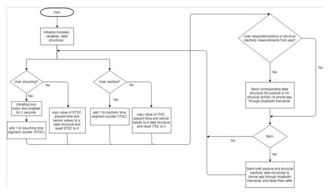
Figure 7: Device Flowchart
