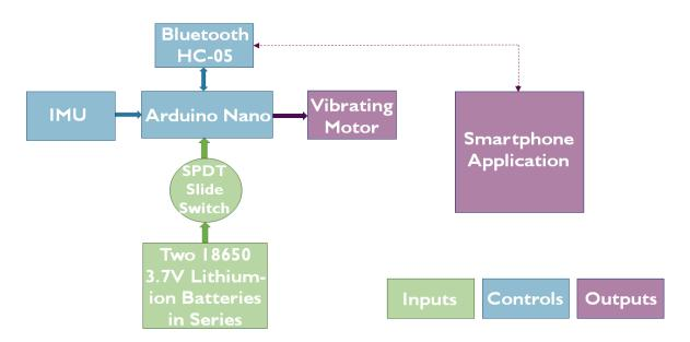
Figure 10: Technical Block Diagram
